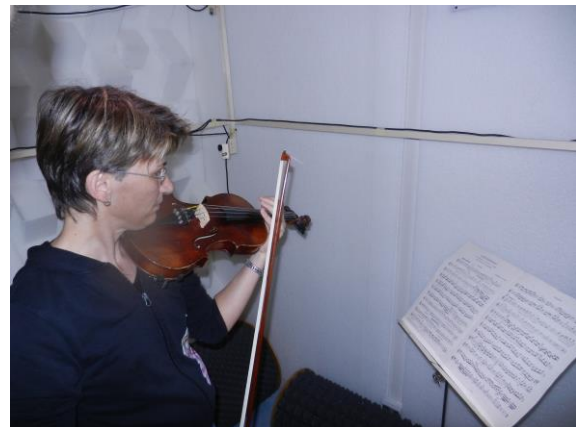
Figure 17: Violin player inside a small anechoic room, surrounded by 8 microphones
