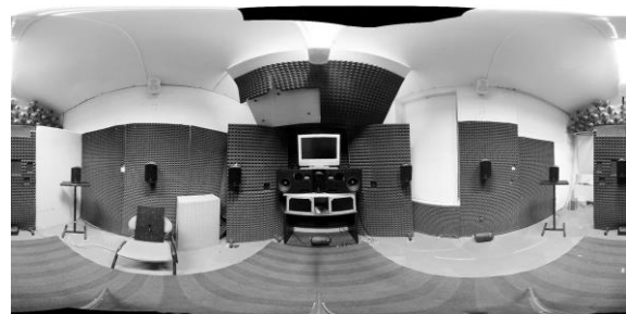
Figure 18: Listening room with 16 loudspeakers
