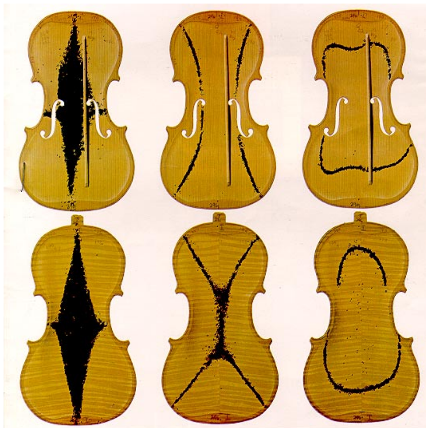
Figure 11. Chladni patterns for violin top and back plates (Cover of Scientific American Magazine, October 1981)
