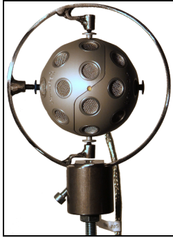
Figure 10: movable fixture for azimuth rotation
