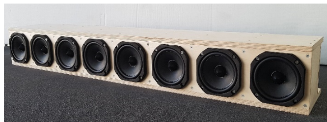
Fig. 10. The 8-channels sound bar of the Wave Field Synthesis system over A 2 B.
