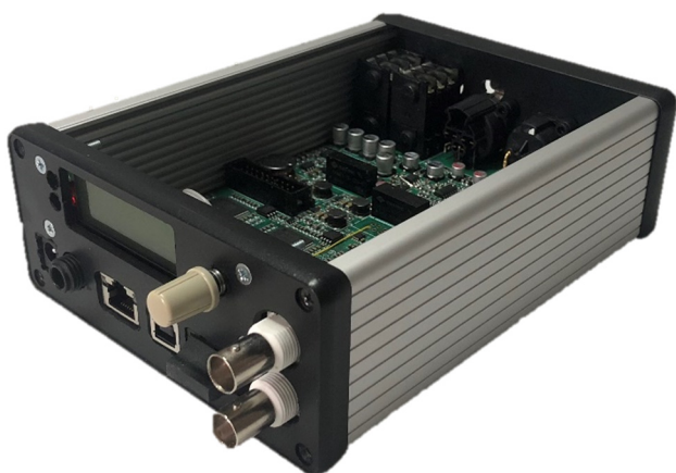
Fig. 8. A picture of the A 2 B-DSP board prototype.
