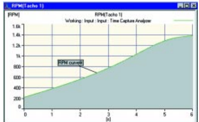
Figure 15. Curvefit of the rpm as a function of time used as input for the Vold-Kalman filtering.
