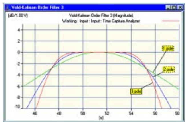
Figure 7. Comparison of the frequency response in the passband for one-, two- and three-pole Vold-Kalman filters with the same bandwidth of 8 Hz.
