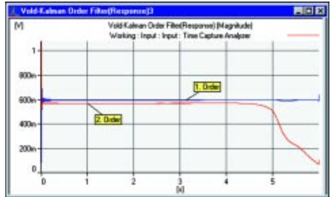
Figure 20. First and second order of the swept signal extracted using decoupling and two-pole Vold-Kalman filter with a bandwidth of 10%.
