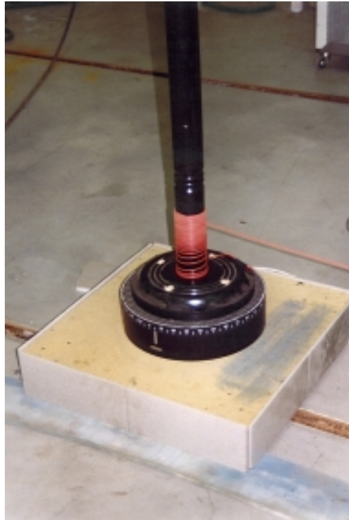
Particular of the rotating board with the cable folding around the drum.
