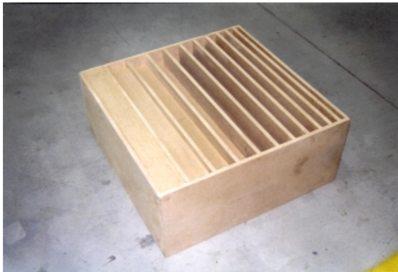
The diffusing panel (named GALAV2) on the reflecting floor.
