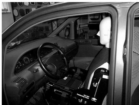
Figure 15 Target car cockpit. Dummy head in the driving position for acoustic measurements.
