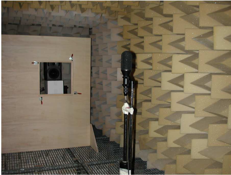
Fig. 17 – The Soundfield ST-250 in the anechoic chamber
