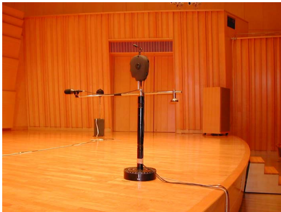
Figure 11: The microphones over the rotating table.
