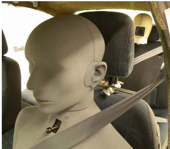
Figure 2 - Head and torso simulator used.
