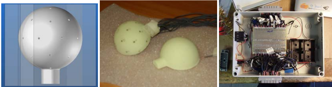
Figure 6.-The CAD drawing of the sphere (a), the two parts of the sphere (b), the self made power pack (c)
