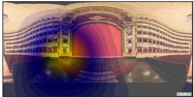
Figure 15 Direct sound in the 4000 Hz band
