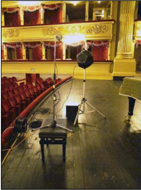
Figure 13 La Scala: receiver in position n.7
