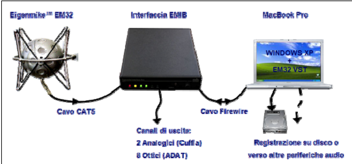
Figure 6 – The complete Eigenmike™ recording system
