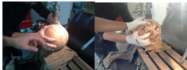
Figure 3 - drilling the 32 holes
