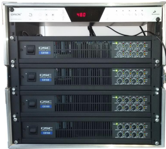
Figure 7 - amplifiers and USB interface, 32 channels
