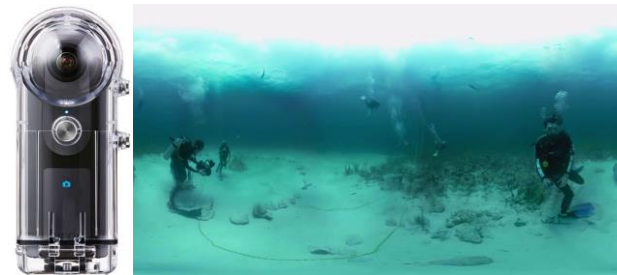
FIGURE 12. UNDERWATER PANORAMIC CAMERA AND RESULTING EQUIRECTANGULAR VIDEO
