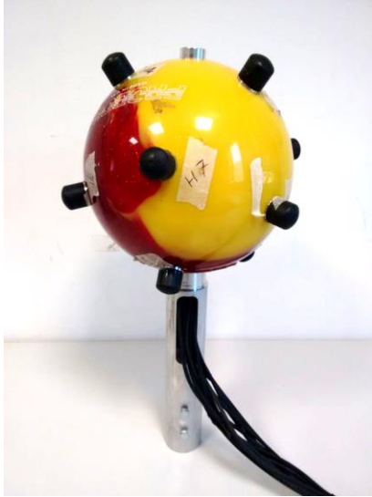
FIGURE 10. A SPHERICAL HYDROPHONE ARRAY WITH 12 SENSORS ON THE SURFACE OF A SPHERE
