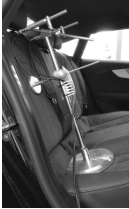
Figure 2: The microphones are positioned on the rear right seat inside the car
