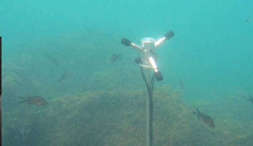
The tetrahedral array of four hydrophones. Credit: University of Parma
