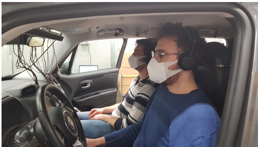
Fig. 5: Two front passengers wearing the binaural microphones (note that the doors were kept closed during the measurements in order to consider a operative condition)
