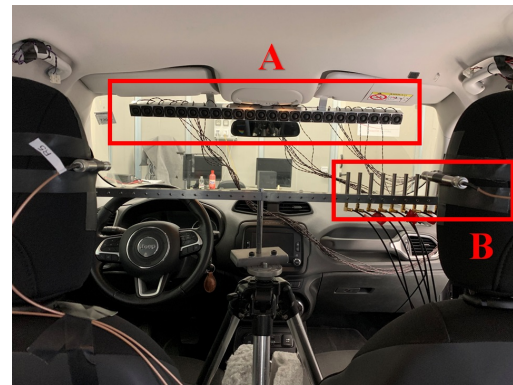
Fig. 4: In-car setup showing (A) the loudspeaker array and (B) the microphone array placed in the dark zone
