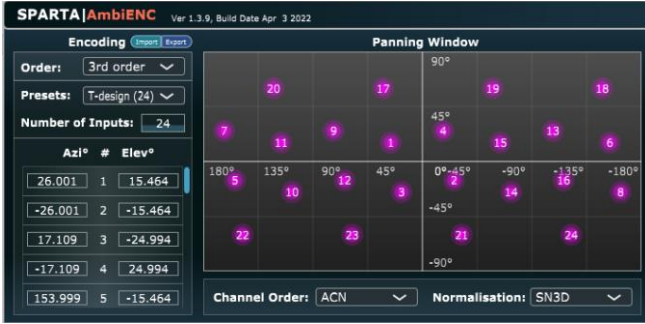
Fig. 16: T-format to B-format conversion using AmbiENC VST plugin.
