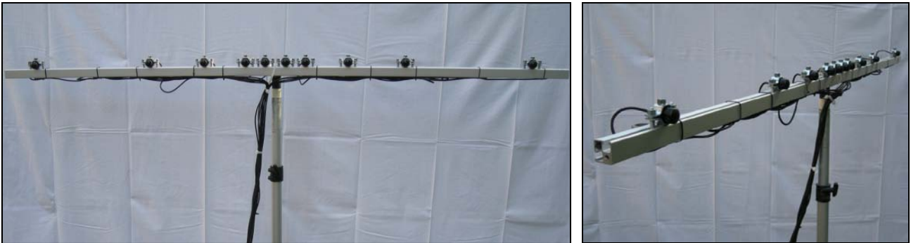
Fig. 1: Ten-hydrophone arranged in the Non-Uniform Linear Array.
