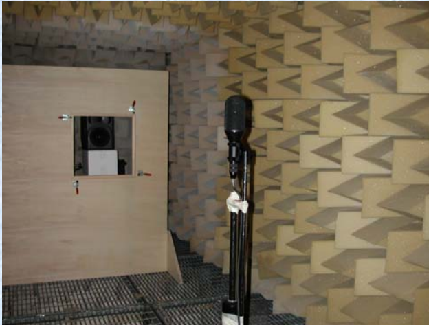
Microphone on the automated rotating table
