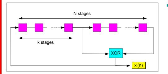
X(t) is a periodic binary signal obtained with a suitable shift-register, configured for maximum lenght of the period.
