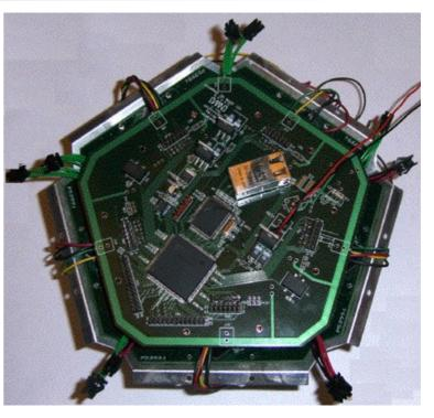
Embedded ethernet interface and DSP processing
