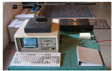
MLSSA was the first apparatus for measuring impulse responses with MLS
