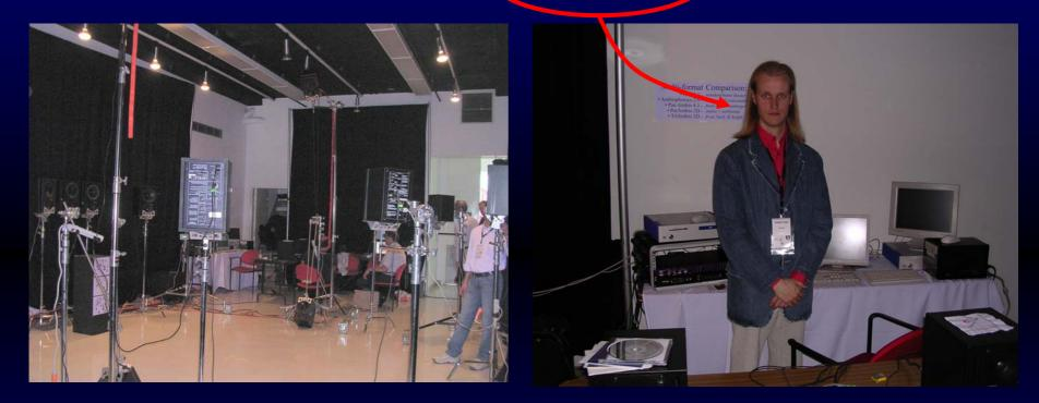
Performance: a fanless (silent) P-IV running at 2.5 GHz was capable of real time convolution of 2 inputs at 44.1 kHz, 24 bits, with 48 impulse responses, each 5s long, driving 24 Genelec loudspeakers (20 satellites + 4 subwoofers), employing 75% of the CPU time
