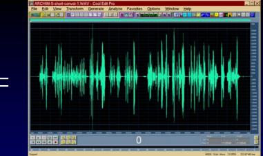
Convolving linearly a suitable sound sample with the Imp.Resp., the frequency response and temporal transient effects of the system can be simulated properly
